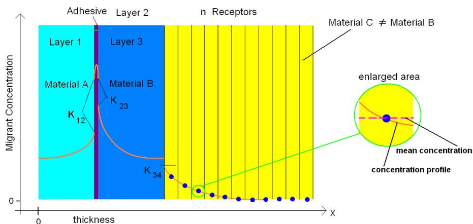
**Figure 4-4: Concentration profile for a substance migrating from the glued sample (Material A and B).**
