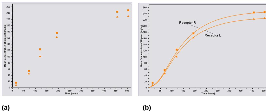
**Figure 4-9: Kinetic experiment: time dependent migration from a multilayer material into a receptor material (a) and migration modelling “Kinetic Method”– best fit between experimental data (points) and calculated data (curve) (b).**
