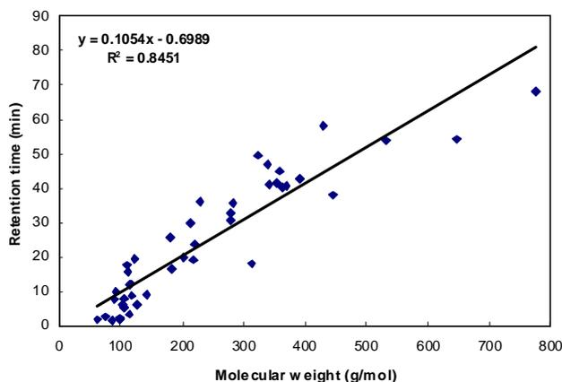
**Figure 4-3: Correlation of the retention time with the molecular weight on GC-FID equipped with DB-1 column.**
