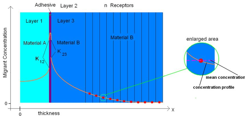
**Figure 4-10: Contamination of receptor material B - concentration profile for a substance migrating from the glued sample (Material A and B)**
