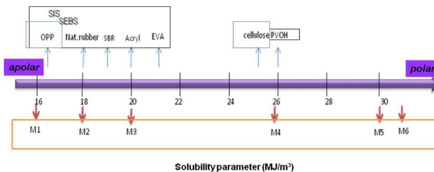
Figure 4-5: Substrates, adhesives and migrants positioned on a polarity scale
