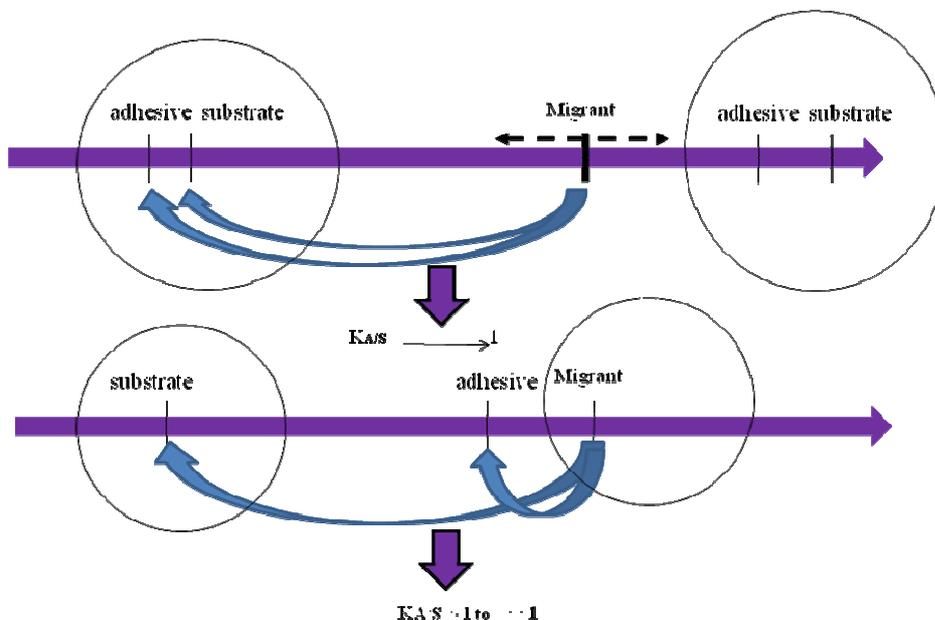
Figure 4-6: : Expected K value as a function of the solubility parameters of the system (substrates and adhesives)
