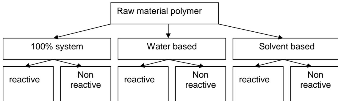
**Figure 4-1: Classification of adhesives according to the raw material polymer, reactivity and solution type**
