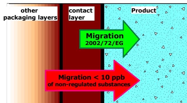
Figure 2-1: Illustration of functional barrier concept in plastic multilayers
