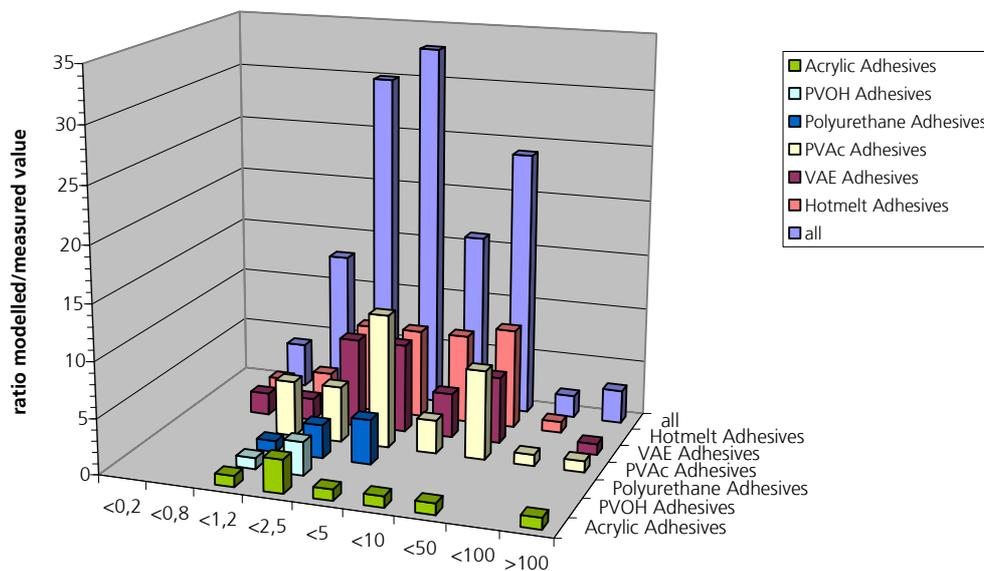
**Figure 4-12: Ratios of calculated versus experimental migration values for migration from 41 laminates onto Tenax, 10 days @ 40°C.**
